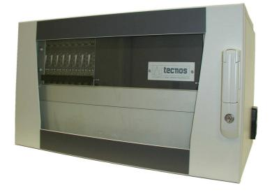
AR600 is the standard case for max. 8 REL/isp modules, ideal for medium size systems or multiple racks systems. AR600 systems are particularly suitable for small areas or on large sites, where it is preferable to have a number of small self-contained monitoring systems connected by a field bus to a remote Host system. AR600 is supplied fully wired, for 8 REL/isp modules and up to 12 ISP alarm outputs with (SPDT) relay rated at 3A 110 Vac.
